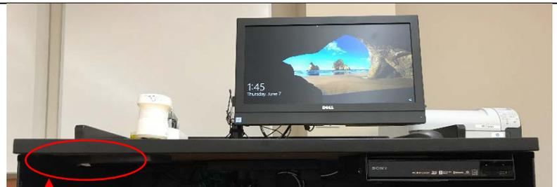
To adjust the height of the console, grasp the adjustment handle and squeeze towards you to release the mechanism. You can then raise or lower the console to desired height.
