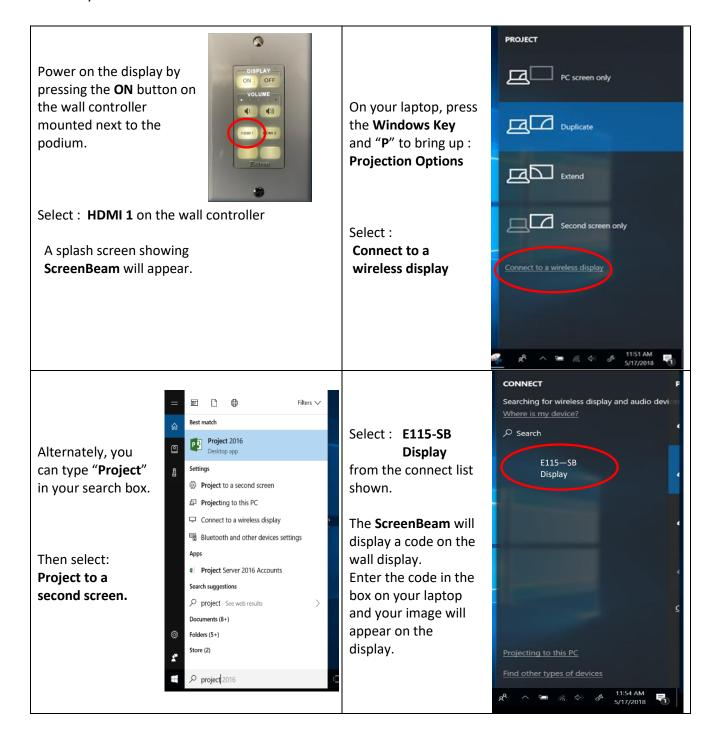
**E115** is equipped with a flat panel LED wall display, an Audio/Video control system and a wall mounted camera with microphone that can be used for web conferencing.
