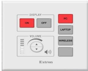
If you wish to connect other devices to the projector, use the **Laptop** cable at the station and press the **Laptop** button on the controller. Adapters for most model laptops are attached to the Laptop cable.
