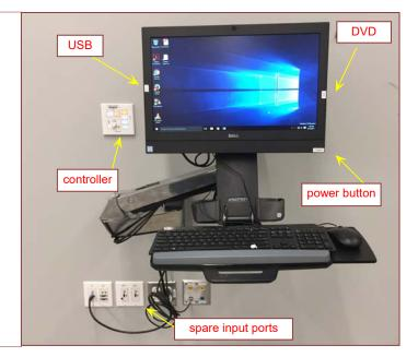
The **USB** ports are located on the left side of the computer screen. There are spare input ports below the arm mount that correspond to buttons on the wall control for additional devices such as a laptop or media players.
