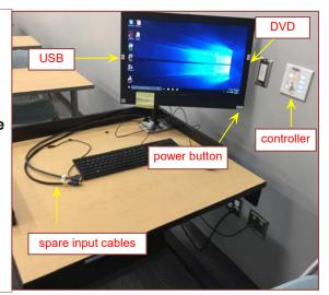
The **USB** ports are located on the left side of the computer screen. If you wish to connect other devices to the projection screen, use the cables on top of the console and press the corresponding button on the A/V controller.
