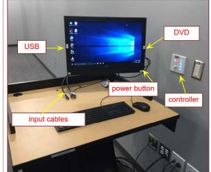
The **USB** ports are located on the left side of the computer screen. If you wish to connect other devices to the projection screen, use the cables on top of the console and press the corresponding button on the A/V controller.
