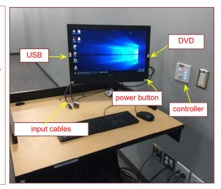
The **USB** ports are located on the left side of the computer screen. If you wish to connect other devices to the projection screen, use the cables on top of the console and press the corresponding button on the A/V controller.
