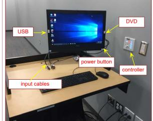
The **USB** ports are located on the left side of the computer screen. If you wish to connect other devices to the projection screen, use the cables on top of the console and press the corresponding button on the A/V controller.
