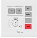
the **Laptop** button on the controller. Adapters for most model laptops are attached to the HDMI cable.
