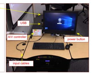
If you wish to connect other devices to the projection screen, use the cables on top of the console and press the corresponding button on the A/V controller. The **USB** ports are located on the left side of the computer screen.
