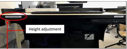
To adjust the height of the console, grasp the adjustment handle and squeeze towards you to release the mechanism. You can then raise or lower the console to desired height.
