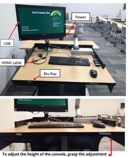
To adjust the height of the console, grasp the adjustment handle and squeeze towards you to release the mechanism You can then raise or lower the console to desired height.
