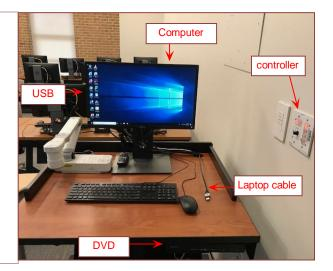
The **USB** ports are located on the left side of the computer screen. If you wish to connect other devices to the projection screen, use the cable on top of the console and press the corresponding button on the A/V controller.
