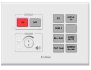
**HDMI 2** button on the controller. Adapters for most model laptops are attached to the HDMI cable.
