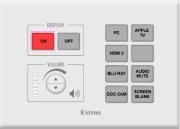
**HDMI 2** button on the controller. Adapters for most model laptops are attached to the HDMI cable.
