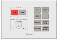
and press the **HDMI 2** button on the controller. Adapters for most model laptops are attached to the HDMI cable.
