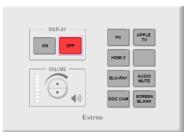
**HDMI 2** button on the controller. Adapters for most model laptops are attached to the HDMI cable.
